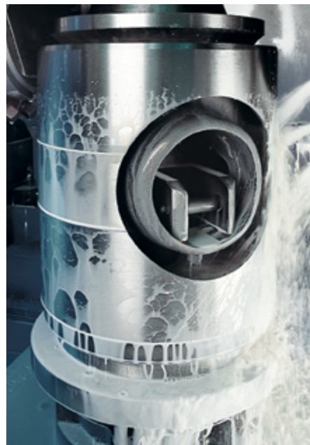
Large bore piston manufacturing with BECHEM Avantin
