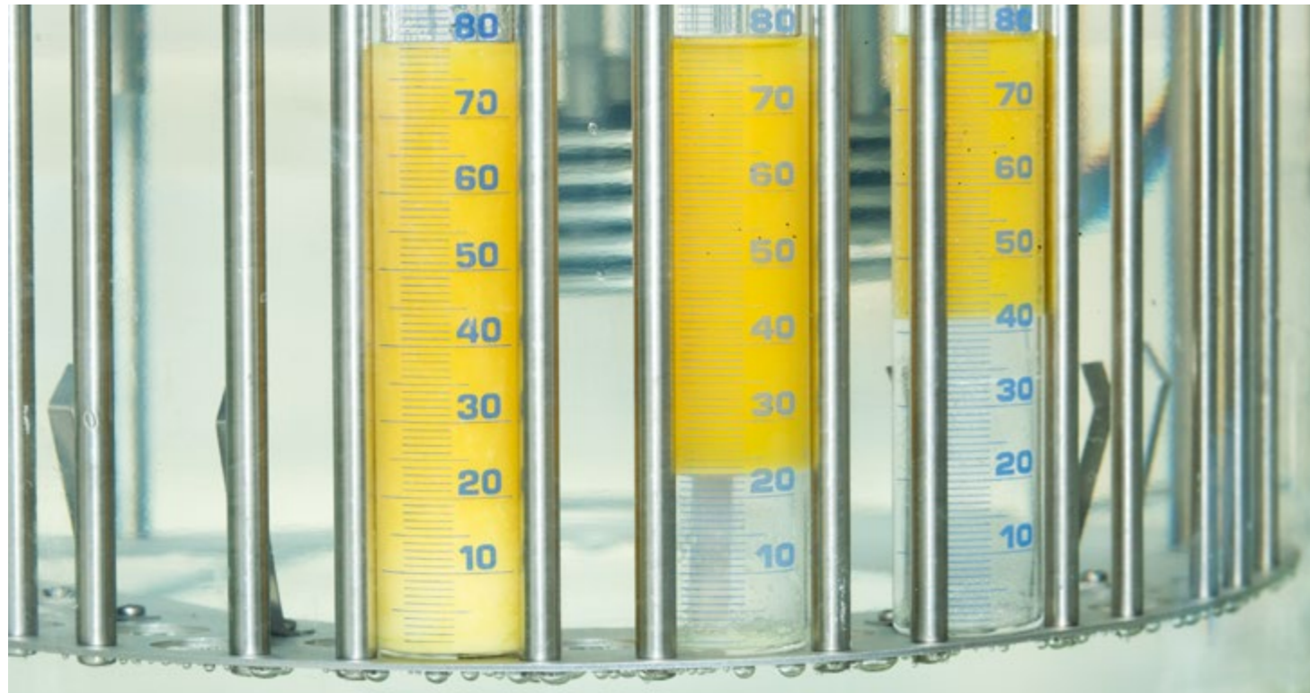
The laboratory test shows the water separation capability of various lubricating oils after five minutes. To the left is the non-optimized, commercially available circulating oil with process water. In the middle is standard oil with process water and to the right is the BECHEM Ovitol KT 460 S optimized for the process water with an outstanding water separation value.
